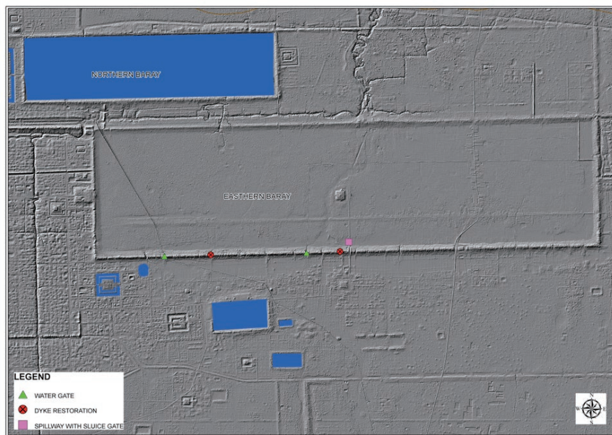
Figure 5.8.1: The restoration South dike of East Baray to bring back water like in the 9 th century
